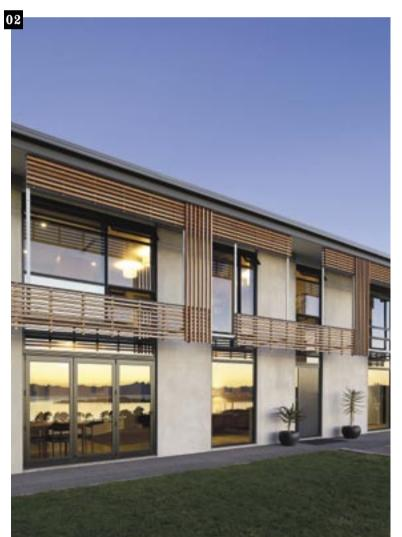
rchitects often explore and exploit the boundaries emplaced by the restrictions of building, and Jeremy Smith has followed suit through the design of the Tilt Panel House. Concrete tilt panel construction, which is often a commercial approach to fabricating buildings, was used by Smith as a way to provide a durable, cost efficient and thermally sustainable solution for the four bedroom family house on a new suburban subdivision in Nelson.
